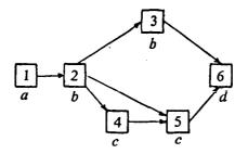
Notice that this node-labelled graph can not be a dep-graph of any trace over any dependency on X. The reason is that the occurrences of c depend on the first occurrence of b, but are concurrent with the second occurrence of b.
