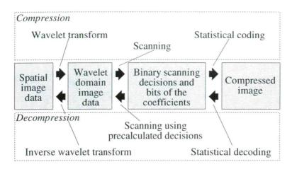
Figure 1: The structure of the DLWIC compression algorithm
