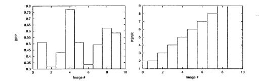
Figure 6: All the images of the test image set are compressed by JPEG with the same quantization value (20), and the BPP (left) and the PSNR (right) of the resulting images are shown.
