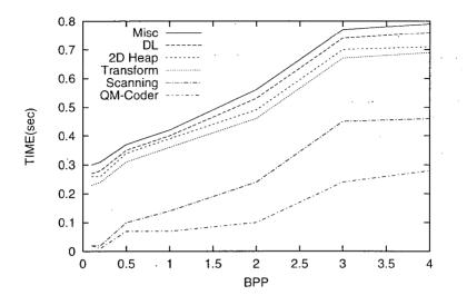
Figure 7: Running time of the different components in the DLWIC compression/decompression algorithm, when compressing the frog test image (Fig. 4). Graph shows the cumulative CPU time consumption when different BPP-rates are used.
