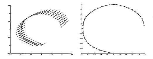
Figure 2: Stratified motion planning for hexapod robot: *i*) constant orientation,  $\theta = \frac{\pi}{3}$  radian (left); *ii*) tangent orientation; "o": reference points, "+": reached points (right)
