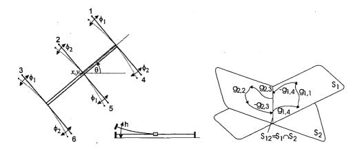
Figure 1: The hexapod robot (left); A tripod gait in the stratified configuration space of the hexapod robot (right)
