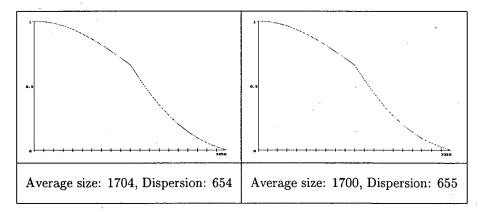
Figs 9-10. The oversize distribution functions shown at the outlet of the mill after t=66 and t=76 units of time, respectively. Continuous grinding without recirculation.
