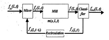
Fig.A. Continuous grinding system with classification and recirculation
