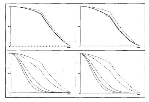
Figs 13-16. The oversize distribution functions shown in the first, third, tenth, fifteenth and twentieth columns of the mill at  $t=5^{th}$ ,  $t=8^{th}$ ,  $t=150^{th}$  and  $t=287^{th}$  units of simulation time. Continuous grinding with recirculation. Discrete model number I. Parameters: I=20, J=20, m=2, n=2,  $V_F=0.3$ ,  $V_B=0.1$ ,  $L_{max}=5000$ ,  $K_s=10^{-8}$ , d=4.
