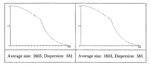
Figs 11-12. The oversize distributions shown at the outlet of the mill after t=1143 and t=1153 units of time, respectively. Continuous grinding with recirculation.
