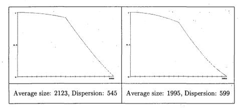
Figs 3-4. The oversize distributions of the particulate product at the outlet of the mill after t=10, t=20 units of time, respectively. Continuous grinding without recirculation. Discrete model number I. Parameters: I=20, J=20, m=2, n=2,  $V_F=0.5$ ,  $V_B=0.1$ ,  $L_{max}=3050$ ,  $K_s=9\cdot10^{-9}$ , d=4.
