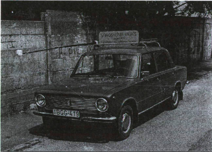
Fig. 3 The measurement car with the temperature sensor (under the white cover)
