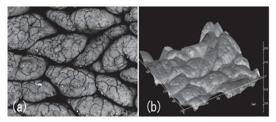
Figure 1A, 1B. A result of 3D observation by our 3D-SEM is shown in the figure below ((a) secondary electron (SE) image, (b) 3D-image obtained through four BSE detectors. Sample: rat intestinal villi). Measurement accuracy increases successfully, because some important improvements have been performed.
