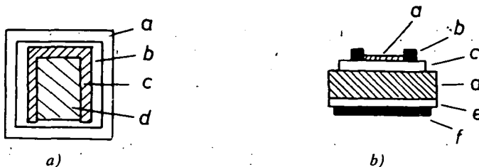
Fig. 1a. Front side of the samples: a free silicon surface; b free vanadium pentoxide surface; c gold electrode of 3 \mu thickness; d semipermeable gold film of about 500 \text{ \AA} thickness.
