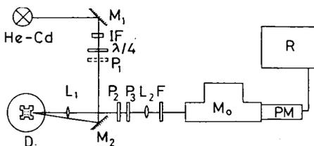
Fig. 2. Diagram of the set up for the determination of the fluorescence polarization ratio. He-Cd, laser for the excitation;  $M_1$ — $M_2$ , mirrors; IF, interference filter;  $\lambda/4$ , quarterwave plate;  $P_1$ — $P_2$ — $P_3$ , sheet polarizers; S, sample holder; D, dewar;  $L_1$ — $L_2$ , lenses; F, cut-off filter; Mo, monochromator; PM, photomultiplier; R, chart recorder
