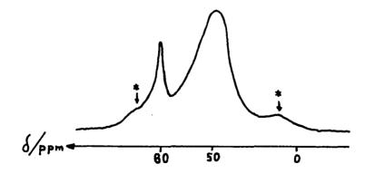
Fig. 1. <sup>27</sup>Al MAS NMR spectrum of the 300DB-sample, partially rehydrated, measured at 70 MHz, \* denotes spinning side bands.
