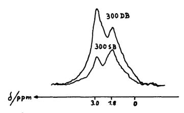
Fig. 2. <sup>1</sup>H MAS NMR spectra of dehydrated 300DB and 300SB samples, measured at 270 MHz
