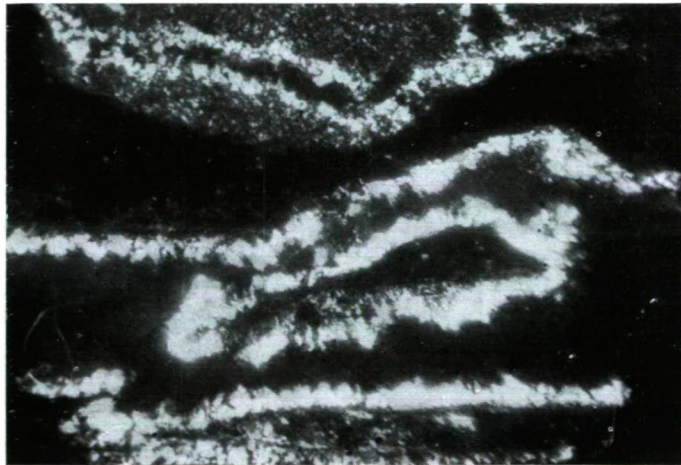
Fig. 5. Fissures filled with heulandite in andesite tuffite. Crossed nicols, 40×
