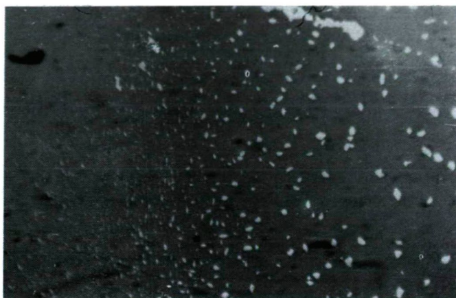
Fig. 1. Ex-solution structure of chalcopyrite in sphalerite from Murgul, Artvin vilayet. Magn. 160 x
