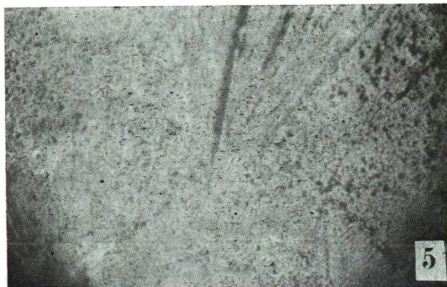
Fig. 5. Radiating structure of pyrolusite developing from the cryptomelane banding. Sandur, Karnataka. Polished section, \times 70
