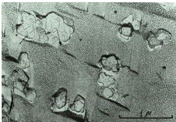
Fig. 2. "Etching pits" on microcline surface and aggregates of kaolinite crystals growing on it. Eleninskoe kaolin deposit, Ural Mts.
