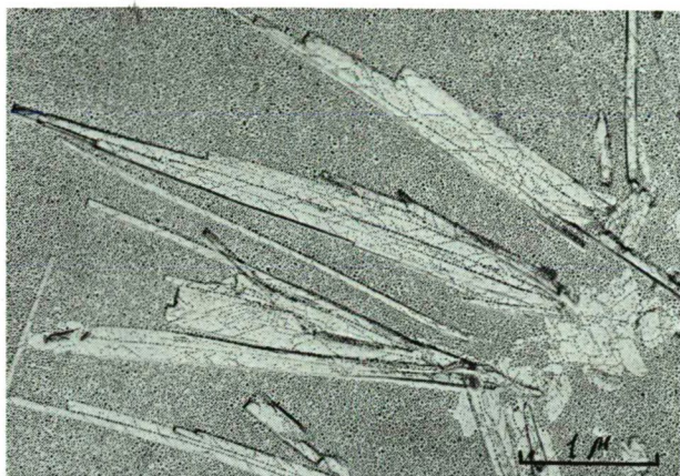
Fig. 3. Platy and tubular halloysite (7 Å?) crystals on the surface of weathered oligoclase. Soyuznoe kaolin deposits, Ural Mts.
