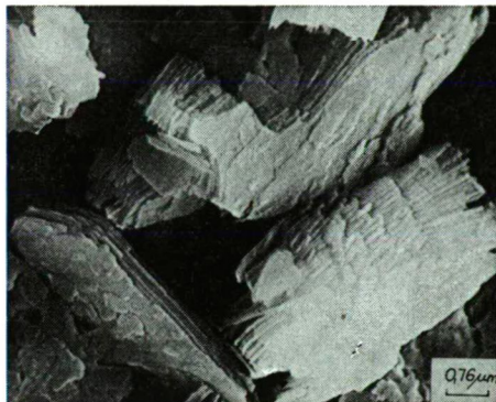
Fig. 2. Particles in the aqueous suspension of Sedlec (Zettlitz) and OKA kaolins
