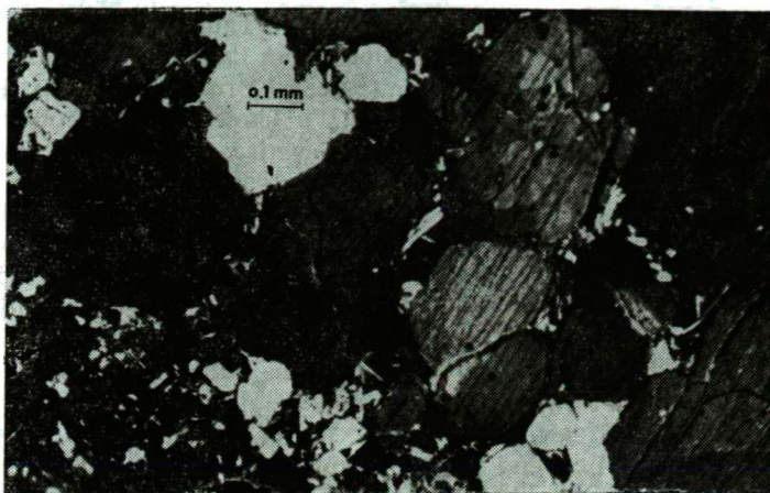
Fig. 4. Photomicrograph showing development of subgrains in an olivine xenocryst from the Nógrád-Gömör region. Crossed nicols.
