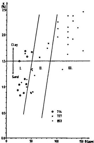
Fig. 12. Chemofacies-analysis of the clayey beds (Clay) and of the grained over- and underlying formations (Sand) from boreholes 714., 727., and 853. on the basis of the K/B ratio. I.=eolic, II.=fluvialitic, III.=lymnic (paludal) sediments.
