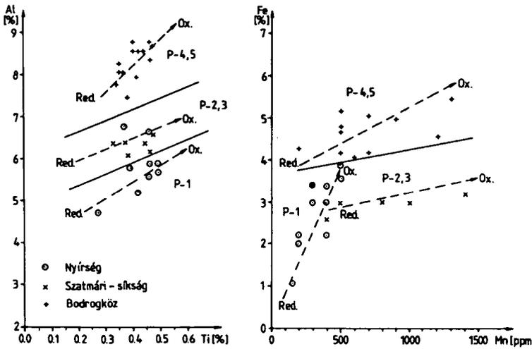
Fig. 11. Correlation between Al-Ti and Fe-Mn element pairs on the basis of the study of low-carbonate ( $\text{CaCO}_3 < 3\%$ ) pelitic sediment from NE Tiszántúl (Transtibiscia). P-1, P-5= subfacies, oxidative (Ox.) and reductive (Red.) environments.
