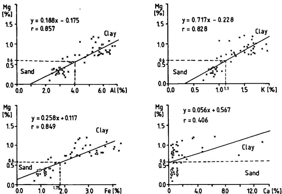
Fig. 10. Correlation between Mg and Al, Fe, K, Ca on the basis of the study of pelitic sediments (Clay) and grained over- and underlying beds (Sand) from boreholes of the section Hajdúdorog-Tiborszállás.
