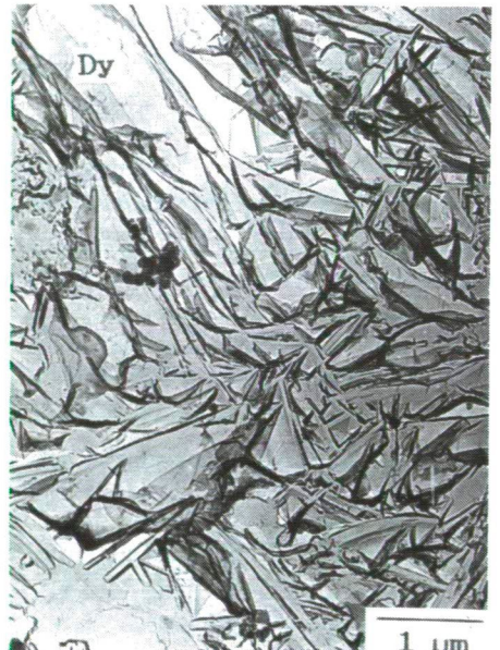
Fig. 8. TEM photograph of dypingite crystallites terminated by (hk0) (hkl) planes. Some clusters of alpha-sulfur (S) can also be seen.
