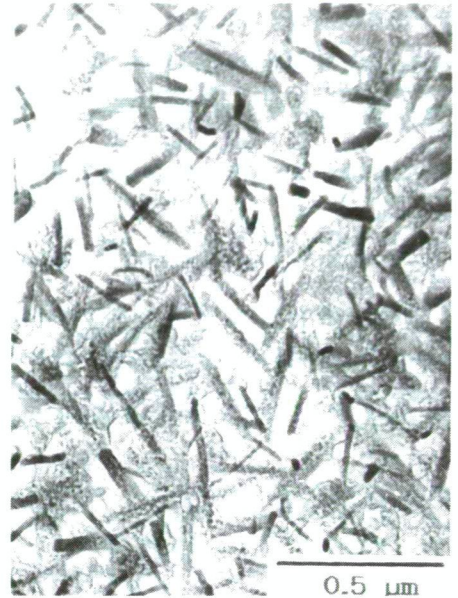
Fig. 14. TEM photograph of some feather-like palygorskite (Pa) crystallites. Acid insoluble residue of a calcite-aragonite dripstone.
