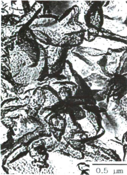
Fig. 7. TEM photograph showing the resorption-recrystallization formations of the single phase nesquehonite (Ne).
