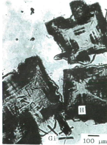
Fig. 20. Microphotograph of powder-like halite (Ha) and gypsum (Gi) precipitation on the surface of a nesquehonite ooid. The outer edge of the halite crystals showing decreescence is slightly brownish coloured and anisotropic (=H hydrohalite (?)).
