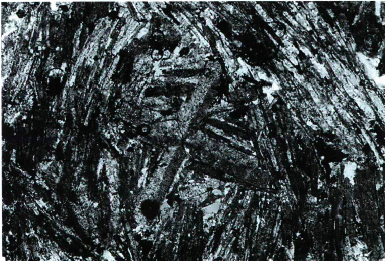
Fig. 4. Sanidine penetration from Mórágý quarry. 100x, +N.
