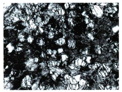
Plate 1/1. Very fine grained symplectitic texture of the Szarvas-16 eclogite with erroded garnet grains.
