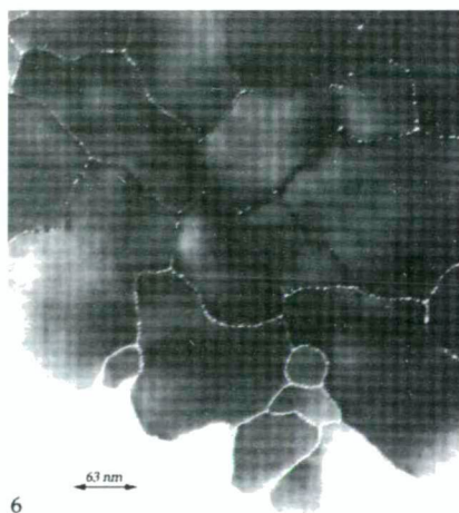
Fig. 4. TEM micrograph of a szaibelyite bundle in cross section
