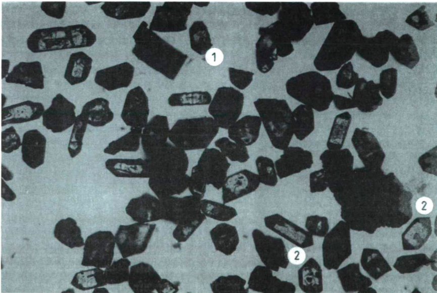
Fig. 1: Zircons from ÁGK-6839 sample under microscope 10x, |N; 1. zircon with inclusion of earlier stage, 2. magnetite inclusion in zircon.
