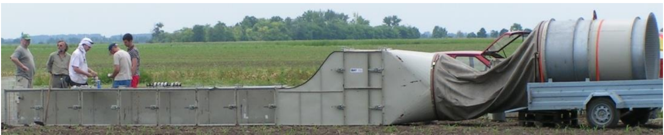
Fig. 4 The portable wind tunnel
