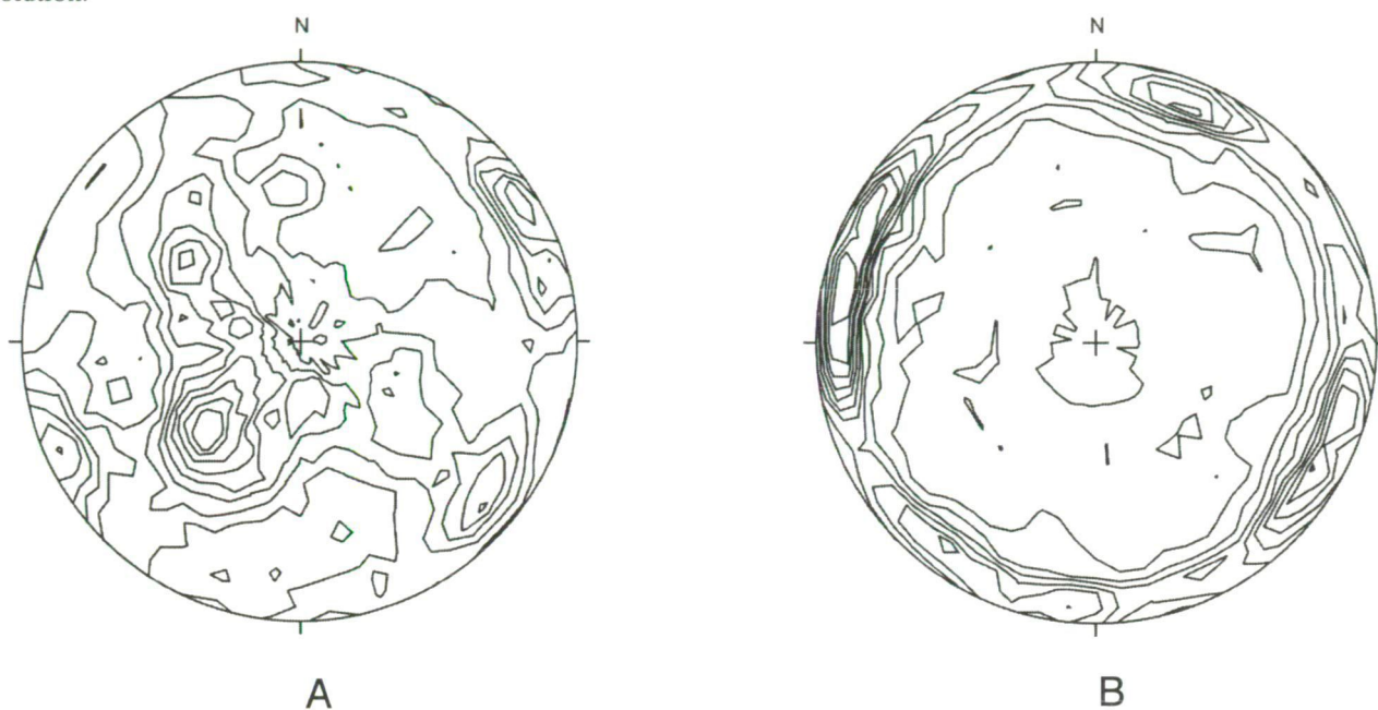
Fig. 1: A) Contour diagram of poles of the fractures from the PTP-3 borehole from depth 20 -348 m (lower hemisphere polar, equal area, number of points = 877) B) Contour diagram of poles of the FIP from the PTP-3 borehole (lower hemisphere polar, equal area, 17 samples, total number of points = 1554)
