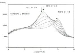
Fig. 1: Comparison of basal 001 diffractions during dehydration of different ionic forms of smectite. Diffractograms were obtained with temperature steps of  $5^{\circ}$ C in the range  $25-300^{\circ}$ C
