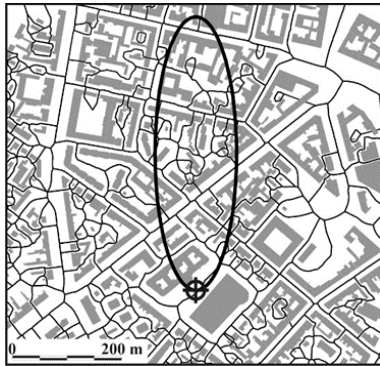
Fig. 7 Illustration of the fetch in an urban area (the cross shows the measurement site)
