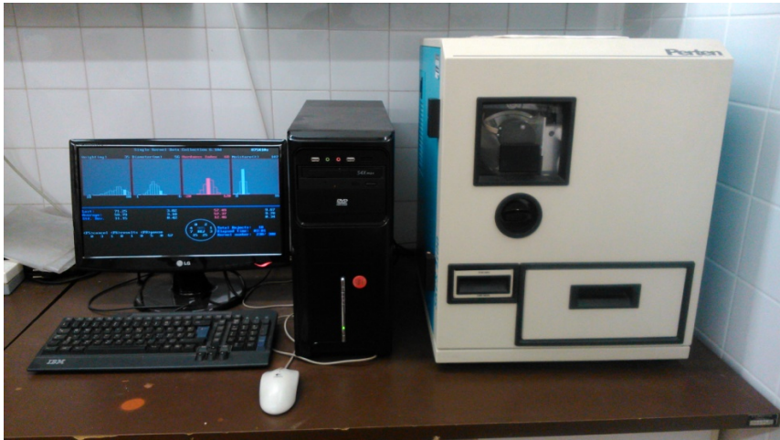
Figure 2. Perten SKCS 4100 machine (Perten Inc)
