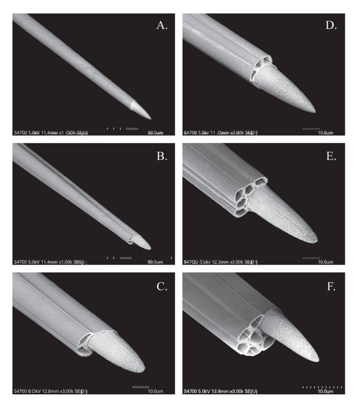
Figure 1. Scanning electron micrographs of carbon fiber microelectrodes. Single-barrel microelectrodes are consisted of a conical carbon tip protruding from the borosilicate glass insulation (A). A varying number of micropipettes can be attached to the recording carbon fiber containing barrel (B-F) for delivering drugs by microiontophoresis or pressure. Filling of the drug barrels is facilitated by inner glass microfilaments fused to the inner wall of the microcapillaries (F).
