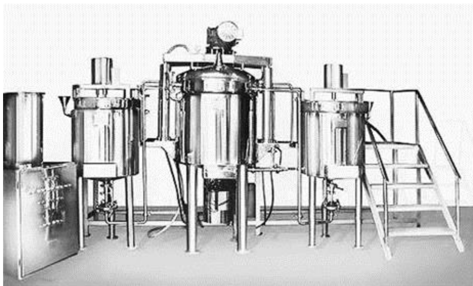
Figure 2. Industrial ointment producing equipment (Source: The Basics of Pharmaceutical Technology, Dévay A. (2013.) [5])
