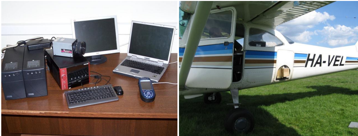
Fig. 1 Hardware elements of the recording system (left) and the Cessna 127 airplane with the CIR camera fixed into its luggage space (right)
