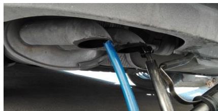
Figure 1: Picture showing connection of the pipes to the car exhaust
