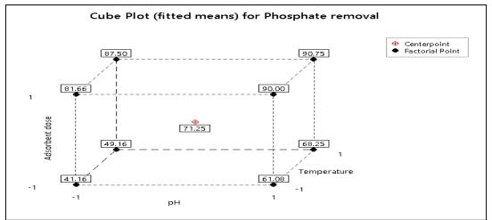
Figure 1. Cube plots for PO<sub>4</sub><sup>3-</sup> removal by IL-PP
