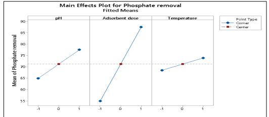
Figure 2. Main effects plot for PO<sub>4</sub><sup>3-</sup> removal by IL-PP
