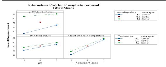
Figure 3. Interaction plot for PO<sub>4</sub><sup>3-</sup> removal by IL-PP
