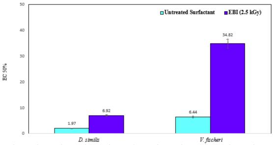
Figure 1. Acute toxicity (EC50% values) of anionic surfactant versus applied EBI dose.
