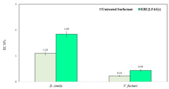
Figure 2. Acute toxicity (EC50% values) of nonionic surfactant versus applied EBI dose.
