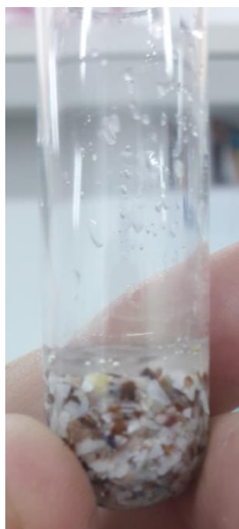
Figure 1. Glass tube containing a sample of shells, fraction 1-1.6 mm, and the phosphorus precursor solution, before the experiment
