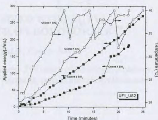
Figure 4. Variation of ultrasonic energy and temperature, applied to the system during synthesis for UF1-US sample
