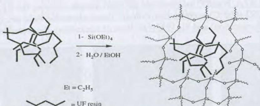
Figure 1: Schematic representation of encapsulated nano-micro-sized UF particles inside silica, hybrid material [3]
