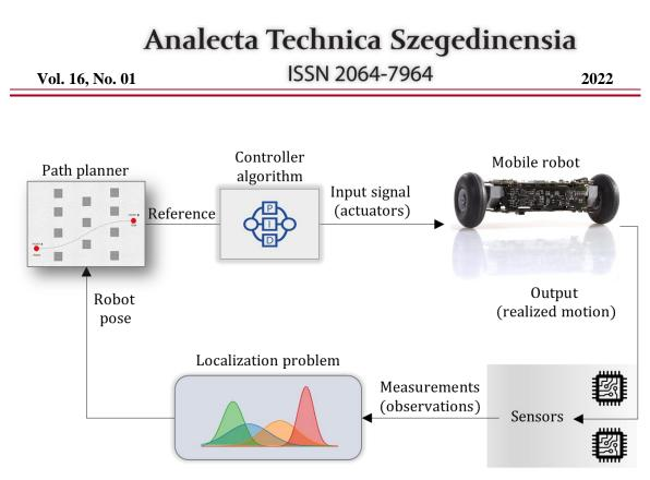
Figure 1: The control structure of mobile robots
