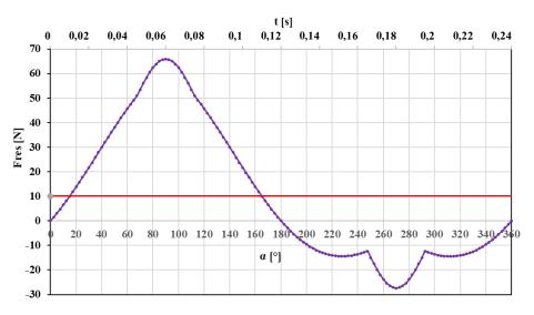
Figure 5. Variation of the propulsion force during a complete rotation of the driving shaft
