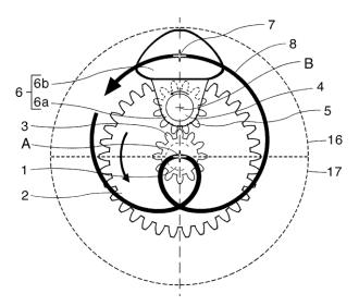
Figure 1. Principle of device for providing propulsion force [2]
