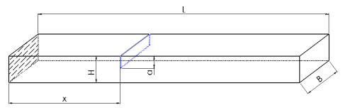
Figure 1. Main dimensions of the cantilever beam
