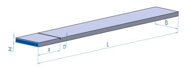
Figure 3. Cantilever beam affected by a transverse crack and weak clamping
