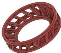
Figure 2. 3D printed spacer used in experiments
