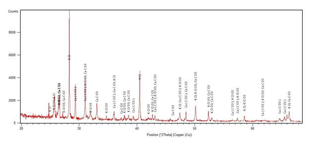
Figure 1. XRD pattern of a sample of shells and sugar/KClO3 mixture after combustion
