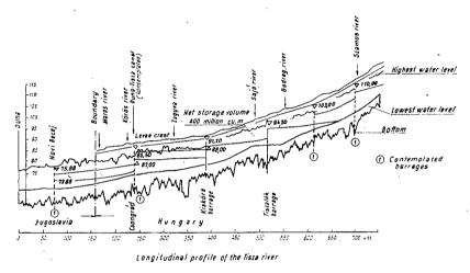
Fig. 2. Longitudinal section of the Tisza canalization
