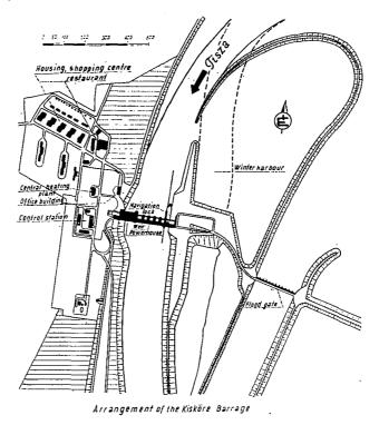
Fig. 4. General plan of the Kisköre River Barrage
