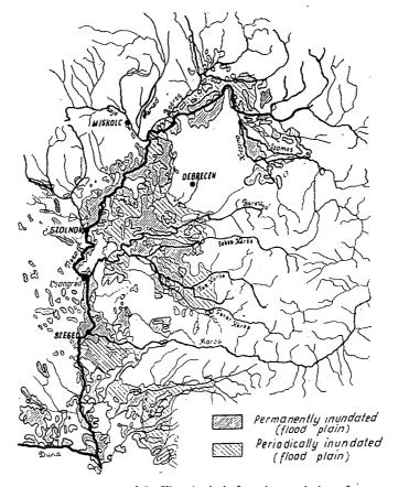
Fig. 1. Hydrographic map of the Tisza basin before the regulation of water-ways
