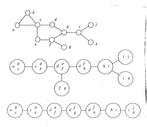
Figure 1. Example of a graph with tree- and path-decomposition
