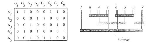
Figure 2. Example of gate matrix layout
