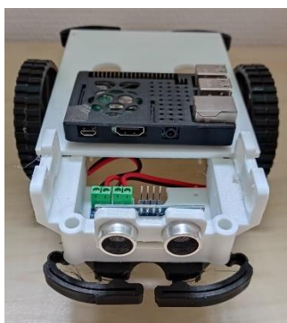
Figure 2. 3D printed and assembled mobile robot platform.
